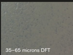
Picture show a polysiloxane topcoat applied with a roller designed for high viscosity, showing the importance of the right application tools to achieve coverage and correct film thickness.
